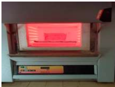
Figure 2. Firing in the SNOL-1200 laboratory furnace
